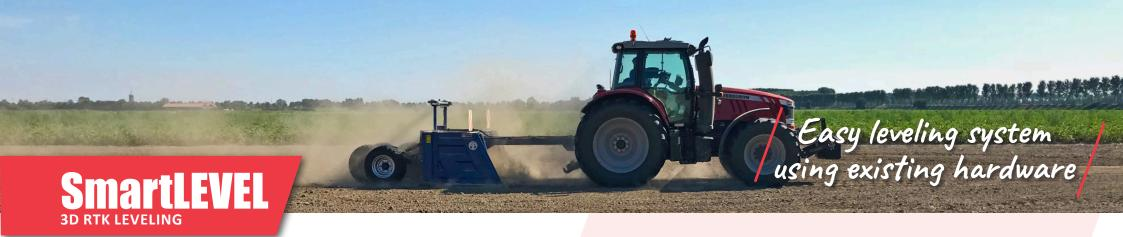
SmartLEVEL leveling/grading for (Ag Leader) ISOBUS RTK systems moves soil all over the world. SmartLEVEL functionality is comparable with laser leveling but grade/slope can be set in up to 3 directions creating double roof model shape. There are unlike laser, no limits in elevation range.
